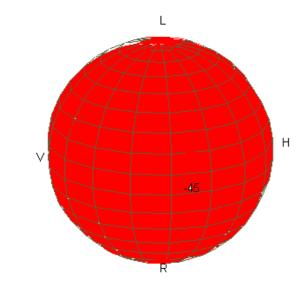
Applying a time varying current to the three sections provides continuous SOP scanning over the full surface of the Poincaré sphere.
