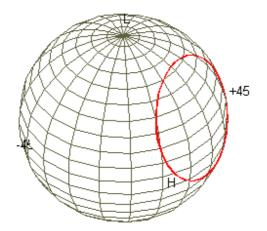
Changing the SOP after the waveplate can move the center of the described circle to any position on the sphere. A change in SOP can be caused by additional birefringent components in the fiber system following the waveplate or birefringence created in the output lead through tight bends or lateral force.
