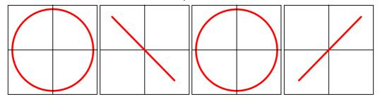
The SOP in the plane of the fiber tail output is dependent on the birefringence of the fiber tail and will be dependent on the temperature. However changes will be on the great circle around the sphere passing through both poles and the equator.
