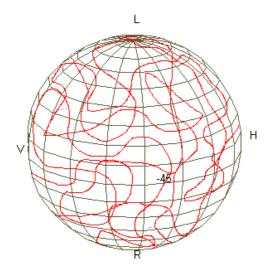
The unit has three current controls and adjusting the current to each of these allows access to any position on the sphere surface from any other position, i.e. conversion of any input SOP to any output SOP.
