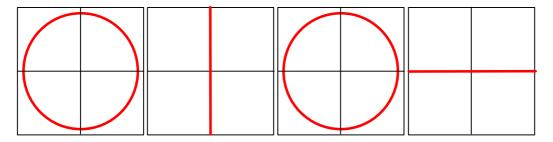
Change of linear output state, i.e. switching between the two axes, can be achieved by switching the drive current.
